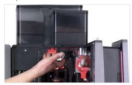
2. Lift and remove the bean hopper.
