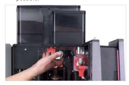
2. Lift and remove the powder hopper.
