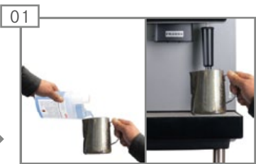
01 Fill container to approx. 5 cm with cold water and 30 ml of clean solution. Place under the steam wand for approx. 1 minute.
